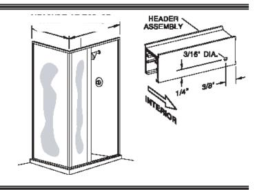
**8** Press the header assembly [**D**] over the wall jambs [**E**] and the 90° post [**K**]. Check the posts for plumb. Adjust as required by varying the overlap of the header over the wall jambs. You may need to trim the ends of the header where it meets the wall. The minimum horizontal dimension for the door opening is the door panel width (see the graphic in Step #9) plus 1/2", maximum is the door panel width plus 1 3/4".
