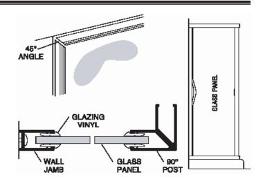
Cut four pieces of the larger vinyl [**KK**] 1/2" longer than the horizontal opening and trim the ends on a 45° angle. Install the top exterior vinyl starting at both ends and working toward the middle. Be careful not to stretch the vinyl.
