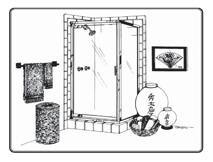
**MAINTENANCE:** Two primary materials are used to manufacture your new Basco enclosure; tempered glass and anodized aluminum. To assure a long lasting finish on the enclosure, wipe it down with a towel after each use. Never use a scouring agent to clean the aluminum.
