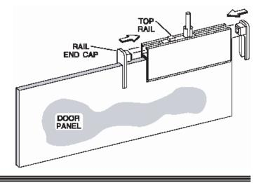
**19** Peel off the backing on the BASCO decal **[HH]** and apply to the inside surface of the header. Trim the flap on the clear vinyl strike jamb seal to clear the bottom door rail.
