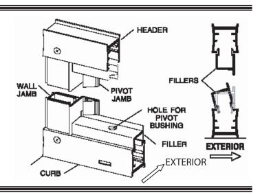
Pull the bottom end of the pivot jamb [**M**] tight to the curb filler [**P**] and plumb the jamb. Drill two 1/8" holes thru the pivot jamb and into the wall jamb [**E**] 3/8" to 3/4" from the wall and approximately 1/4" from the ends of the jamb. Drill a third hole centered between the first two, then enlarge the outer holes with a 3/16" drill for clearance on the self-tapping screws. Attach the pivot jamb permanently with three #8 x 1/4" truss head screws [**C**].
