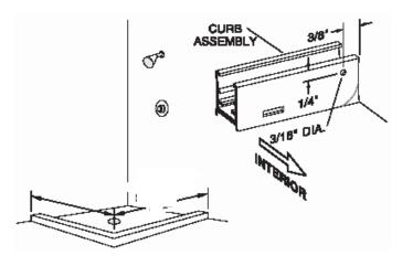
4 Place the two wall jambs [E] into the ends of the curb assembly [A]. Masking tape may be used to hold the curb in place during this operation. Plumb the jambs and mark the hole locations on the wall. Remove all parts and drill the walls for mounting hardware.
