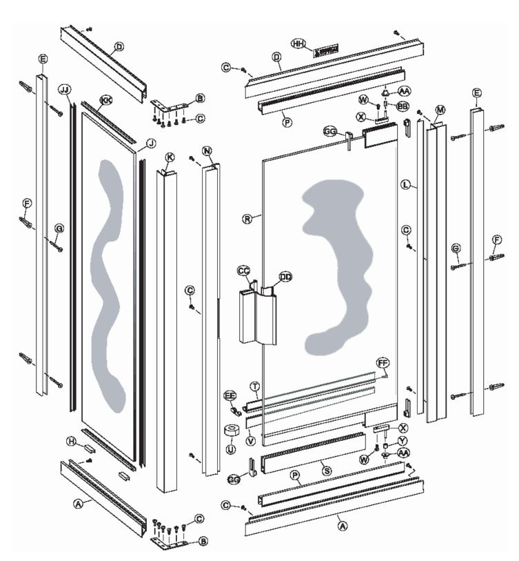
1 Drip Rail 1 Drip Rail 1 Roll Double Stick Tape 1 Tapered Drip Vinyl 2 #10 x 7/16" Set Screws 2 Pivot Blocks
