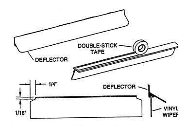
Hold the splash deflector [P] against the inside of the door bottom rail 1/16" from the hinge jamb and with the vinyl wiper [R] just touching the curb. Mark the location of each end of the deflector with a pencil. Peel the backing off of the double-stick tape [S] and carefully (you only get one try) stick the splash deflector to the door using the marks for alignment.
