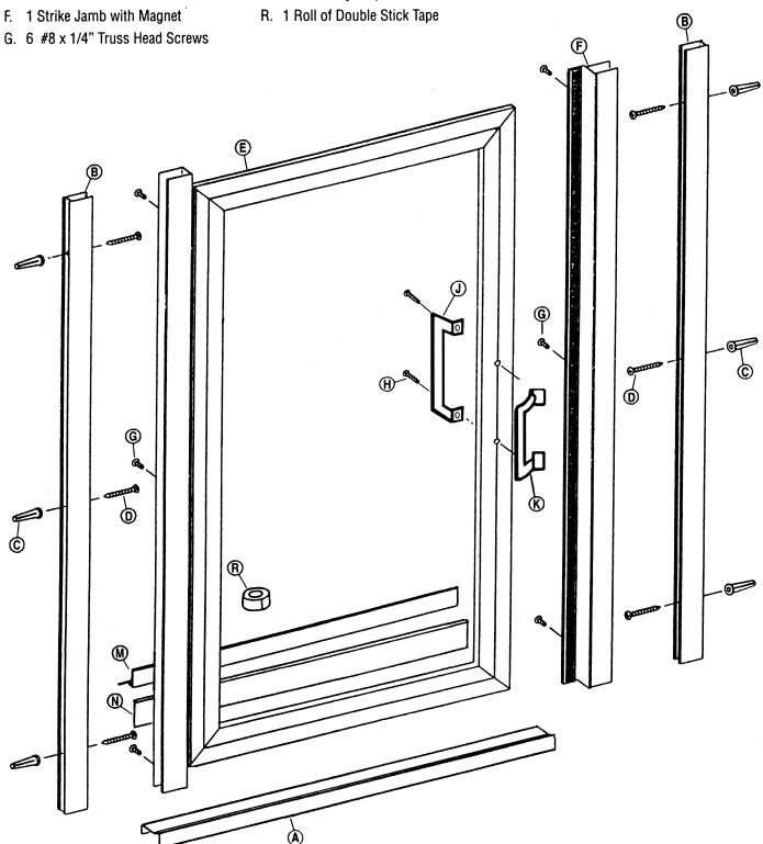
The BASCO 25 Continuous-Hinge Shower Door is completely reversible and may be installed hinge-left or hinge-right. Refer to the illustration to determine the correct position for your installation. For maximum waterproofing, the hinge jamb should always be opposite the shower head. These instructions depict a hinge-left installation.
