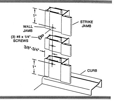
Slide the door panel [E] over the other wall jamb [B] until the door panel and the strike jamb [F] can meet. With the door closed and the latch magnets engaged, the proper door panel to strike jamb clearance is 1/8" (see illustration). Mark the hinge jamb's location on the wall jamb with a pencil.
