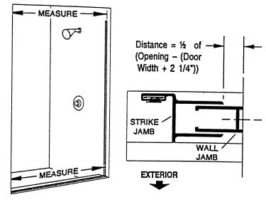
Inside the shower enclosure, drill two 1/8" holes thru the strike jamb [F] and into the wall jamb [B] 3/8" to 3/4" from the wall and approximately 1" vertically from each end of the strike jamb. Drill a third hole centered between the first two, then enlarge the three outer holes with a 3/16" drill for clearance on the self-tapping screws. Attach the strike jamb permanently with three #8 x 1/4" truss head screws [G].
