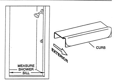
Place one of the wall jambs [B] against the wall with the bottom end 3/16" from the raised side of the curb [A]. Plumb the jamb and mark the hole locations on the wall. Repeat for the other wall jamb. Remove all parts and drill the walls for mounting hardware.
