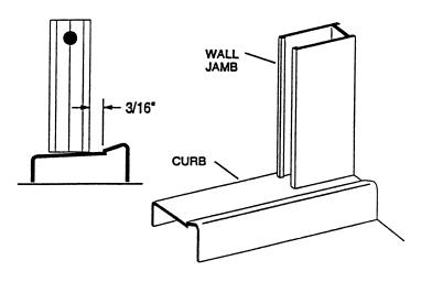
Slide the strike jamb [F] over one of the mounted wall jambs [B] with the magnet facing outward.
