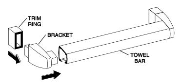
Attach one of the towel bar assemblies (with the open slot in the bar downward) to the interior panel [**B**] with two  $\#10-24 \times 7/8$ " truss head screws [**T**] thru the rails.
