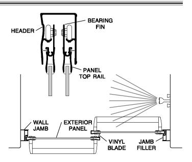
Measure the wall-to-wall opening at the center of the tub rim. Cut the tub track  $[\mathbf{E}]$  1/16" short of this dimension. An inexpensive miter box (available at your local hardware store) will help you get clean square cuts.
