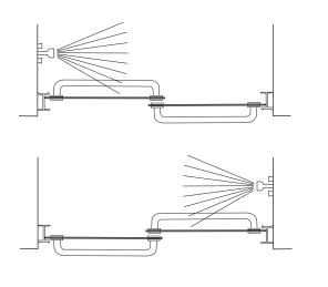
**9** Lift the interior glass panel into position with the rollers engaging the groove in the header [**F**]. Repeat for the exterior panel. If panels are not parallel to their respective wall jambs, remove and adjust the rollers up or down in their slots to compensate.
