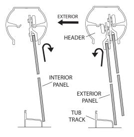
**10** Locate the nylon bottom guide [S] in the middle of the tub track [A] with the glass panels in the position shown. With a 7/64" bit, drill two holes into the V-groove through the mounting holes in the guide. Install the bottom guide with two #6 x 3/8" pan head screws [T] thru the drilled holes as shown.
